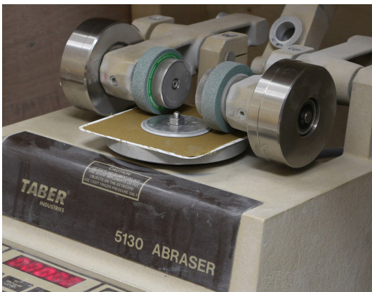
Sample undergoing Taber abrasion test
